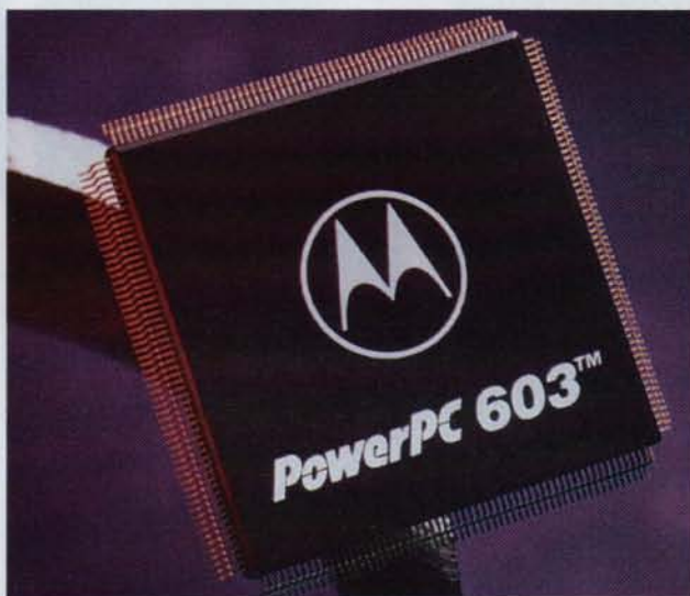
Pippin's CPU will be built around the base-model PowerPC chip, the 603, developed by Apple in conjunction with Motorola and IBM
